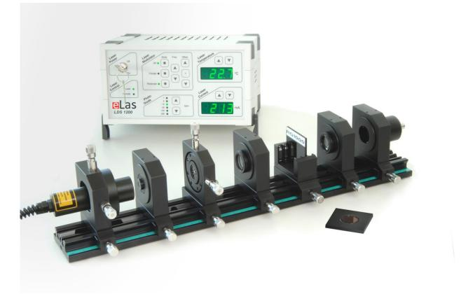
Absorption and emission caused by optical pumping is an important process in solid state lasers. Optical pumping causes the inversion of population necessary for laser operation. The pumping efficiency depends on the choice of proper absorption and emission transitions of the active medium. By tuning the temperature of the laser diode chip a wavelength shift and hence the matching of the laser diode emission with the crystal absorption can be optimized.
