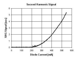
As an example of measurements the second harmonic signal as a function of the pump diode current is shown. The non-linear (quadratic) behavior of the up-converted light can clearly be seen.
