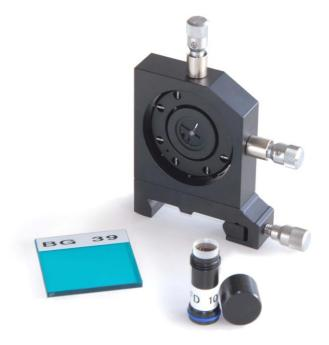
A KTP crystal converts the Nd:YAG emission intra-cavity to green light. For green emission above 5 mW an output coupler mirror highly transmissive at 532 nm is provided. Using an IR-absorbing filter the quadratic response of the SHG process is measured. Transverse cavity modes of the Nd:YAG laser are visualized by SHG impressively.
