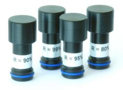
A set of four laser mirrors with reflectivities between 80% and 99% at 1064 nm are provided in this set. The mirrors allow the performance of measurements for which the reflectivity of the mirrors is important. The influence of the reflectivity on the laser threshold and on the slope efficiency is shown. The maximum laser power as a function of the reflectivity is measured. The laser thresholds for different mirrors are plotted and extrapolated for a minimum threshold value.
