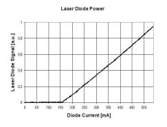
The relative output power of the laser diode used for optical pumping can be measured in dependence on the injection current. Parameters like laser threshold and slope efficiency are evaluated.
