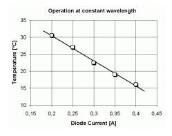
Increasing of wavelength proportional to raising power is characteristic for laser diodes. To compensate this behavior it is necessary to vary its temperature. Operation at a constant wavelength is realized by working at an absorption minimum (i.e. maximum transmission) and optimization of the temperature and current for maximum transmission.
