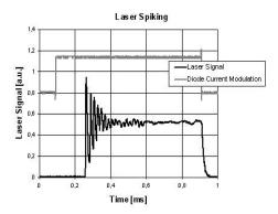
Laser spiking as a result of switching on of the laser is demonstrated. Working close to the laser threshold and in a rectangular modulation mode the effect of spiking and its damping is clearly observable.
