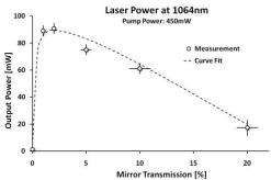
**Extrapolated YAG laser threshold**
