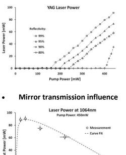
The output power of the Nd:YAG laser can be measured in dependence on the pump power of the laser diode. Parameters like laser threshold and slope efficiency are evaluated for each of the four mirrors.
