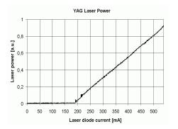
Using the triangular modulation mode of the pump diode current, the Nd:YAG laser power can be presented as a function of the pump diode power. Parameters like laser threshold and laser slope efficiency are determined. Varying the length of the laser resonator, these parameters can be evaluated with respect to the resonator's stability range.
