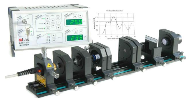
The diode-pumped solid-state laser CA-1230 is a versatile laser source designed for training and educations, but can also be used in research applications. The system with all its extension options (CA-1231 through CA-1234) is the most flexible DPSS system on the market. With its seven operating modes it offers a variety of opportunities for experimentation in the field of diode and DPSS lasers and nonlinear optics.
