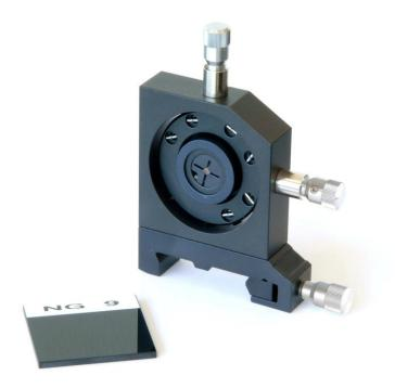
A Cr:YAG crystal acts as a saturable absorber within the resonator. A train of needle like pulses is observed. The pulse frequency is influenced by the pump power and the cavity alignment. When oscillating at more than one transversal mode two or more pulse trains appear. A neutral density filter in the setup avoids saturation of the photo detector. In combination with CA-1231 intra- and extra-cavity SHG can be shown.
