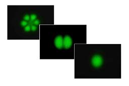
By second harmonic generation transversal mode structures can be visualized. Besides the  $TEM_{00}$  fundamental mode, modes of higher order can be adjusted and determined.
