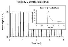
Using the saturable absorber crystal in its 5-axes adjustment holder, passive q-switching is achieved and pulse trains as shown aside are generated. Zooming in a single pulse (insert) its rise and fall time as well as its pulse width of less than 200 ns can be determined.
