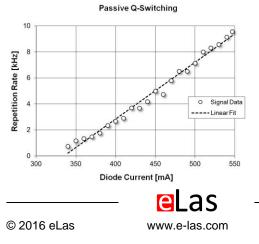
The pulse repetition rate of the passively switched signal can be measured as a function of the pump diode current. As a result one gets a nicely linear behavior.
