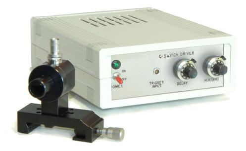
A LiNbO<sub>3</sub> Pockels cell changes the polarization state of the Nd:YAG emission. A Brewster plate introduces losses and laser operation is suppressed. When switching the cell, the losses are minimized and a laser pulse builds up. Periodical switching leads to pulsed laser operation and a q-switched pulse train is observed. Switching voltage and frequency are adjusted by a controller. In combination with CA-1231 intra- and extra-cavity SHG can be shown.
