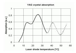
The absorption spectrum of the Nd:YAG crystal in dependence of the temperature of the laser diode is measured. Using the known absorption lines of Nd:YAG the transmitted intensity or the fluorescence intensity of the crystal is measured. By varying the laser diode temperature its emission wavelength is scanned.
