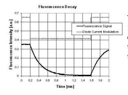
The  ${}^{4}F_{3/2}$  level is the starting level for the emission at 1064 nm. The life time of the fluorescence of the Nd:YAG crystal pumped by the laser diode is detected. The current of the diode is TTL modulated and the decay curve of the fluorescence is measured.
