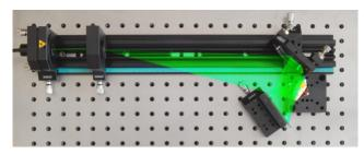
To record a transmission hologram with relatively little effort, a direct beam structure is offered, as shown in the picture. Object and reference beams are formed by one divergent laser beam. The structure is therefore compact, it requires few optical elements and the adjustment effort is limited. As a result, variation options are few only.
