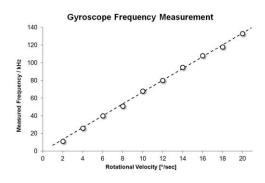
At the beginning of the measurements the scaling factor of the laser gyroscope has to be determined, which gives the relation between the measured signal frequency  $\nu$  and rotational frequency  $\omega$  of the gyroscope. For that the rotation table is driven with a series of increasing angular velocities. The slope of the resulting linear relation gives the desired scaling factor.
