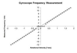
For this measurement one selects a range of small angular speeds and lowers the velocity stepwise. Again, the measured frequencies plotted in a graph as a function of the angular speed result in a straight line which, however, does not go through the origin, but drops at a certain point down to zero. The rotation velocity at which the interference signal disappears is the lock-in threshold.
