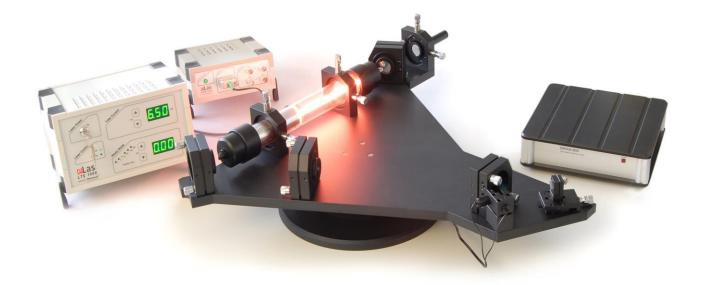
One of the most fascinating applications of lasers is the set-up of a laser gyroscope. This absolute measurement system is a very important tool in daily life: navigation in airplanes and ships, alignment of telescopes, survey of landscapes and high precision rotation measurements to name only a few.
