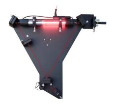
The Laser gyroscope consists of a ring laser which is formed by a He-Ne laser tube and three resonator mirrors. The gyroscope is mounted on a base plate, which can be rotated by a rotating turntable of high precision. The first task of the experiment is to adjust the ring laser and bring the laser to operation. Mode selection is achieved by a single mode etalon, inserted in the ring laser beam path.
