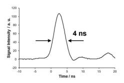
The laser in use is a q-switched laser module with a pulse width of less than 5 ns. With an oscilloscope of 100 MHz or better, the pulse width can be displayed and measured on the oscilloscope screen. It must be taken care, not to saturate the detector. Otherwise the measured pulse width is too large. With its radiation wavelength of 1535 nm the laser is in the eye safe emission region.
