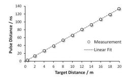
A measurement of time of flight values for a series of distances can be performed. The slope of a linear fit of the data points is related to the speed of light. If big bodies of transparent materials are available, the index of refraction of these materials can be determined (note: the laser emits in the infrared range).
