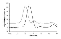
With a pulse width of less than 5 ns, target distances of as short as 40 cm can easily be resolved. Especially for such short distances it must be taken care, not to saturate the measurement detector. A saturated signal may show a pulse elongated by several hundreds of nanoseconds. In the example on the left picture the pulse distance is 2,3 ns which corresponds to a target distance of 35 cm.
