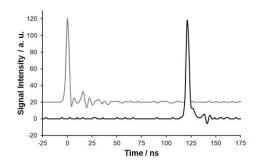
Due to the high peak power and low beam divergence of the laser module, measurements of several tens of meters can be performed. In the example on the left picture the pulse distance is 120 ns which correspond to a target distance of 18 m.
