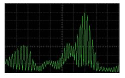
With a frosted disc installed in the rotation stage the detection of permanent LDA signal oscillations are possible, provided the optical system is properly aligned. A signal with quite good signal to noise ratio may look like shown in the scan. Goal is to align the system for a signal with modulation contrast as high as possible.
