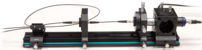
A two channel (red and green LED) transmission line with a short piece of POF is set up. The signal values of the two channels are detected and the attenuation of the two connectors is calculated. The attenuation of the short fiber piece may be neglected in first approximation.
