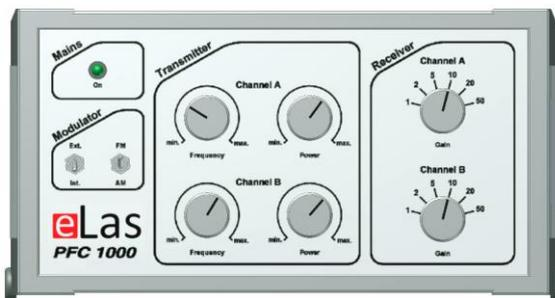
The transmitter and modulator unit of the Plastic Fiber Controller PFC 1000 converts electrical to optical signals which are launched into two plastic optical fiber channels by a red
