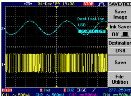
A sinusoidal signal (upper curve) is transmitted in the FM modulation mode like shown in the lower curve. A rectangular TTL signal is modulated in its frequency according to the sinusoidal input signal.
