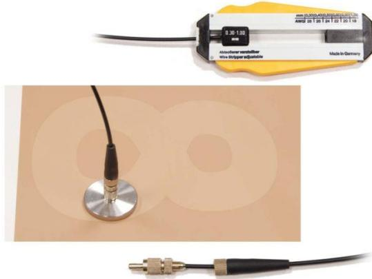
Although the setup comes already with terminated and polished fibers, a set of tools, a bare fiber coil and connectors are added to get experienced to prepare the fiber to be connected and subsequently to be polished. Since the FSMA connectors can be removed easily from the fiber it can be a first task of the students to assemble a pair of connectors to a piece of fiber, as well as grinding and polishing the fiber tip for optimum transmission.
