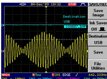
If the two input signals have almost the same frequency, one can observe a signal beating which is the result of alternating constructive and destructive interference of the two signals. This beating is nicely observed if the two signals are detected by one photo detector and the amplitudes of the two signals have the same heights.
