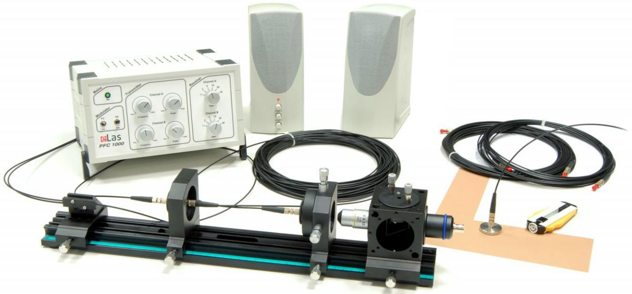
Optical data transmission is nowadays a standard technique in telecommunication. Glass fiber lines are widespread all over the globe. However, in multimedia systems, automotive systems, home networks or control systems plastic optical fiber (POF) networks can often be found. Reasons for the choice of POF can be the lower price, the need of only short transmission lines (50 – 100 m), environmental conditions not suited for glass fiber, or simply the easy way of installation of a POF network.
