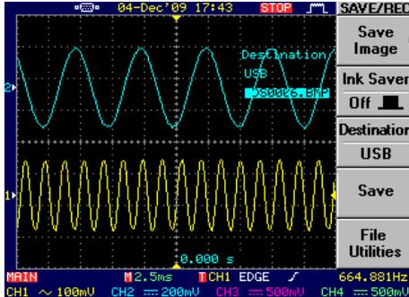
Feeding the two modulated output signals to the oscilloscope the graph may look like the following picture. Here one signal frequency is chosen as about three times the frequency of the other signal.
