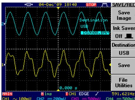
If one signal channel has a much higher amplitude than the other, the effect of cross talk may appear, i.e. the signal of one channel is more or less present at the other channel as well. This behavior is presented in the next graph which shows the “pure” signal from the modulator output in the upper curve and the same signal overlaid by the second channel’s signal from the demodulator output in the lower curve.
