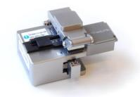
For splicing two fibers, the fiber coating has to be stripped off by the fiber stripper, as mentioned above. Further, the two bare ends of the fibers have to be cleaved by a precision cleaver provided in the kit. After cleaving the fiber ends show a smooth, flat surface.
