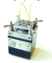
In a next step the connector is grinded and polished. For this task a polishing machine is used. The projecting fiber end is cut off with the ceramics blade. The connector is mounted on the polishing machine. In a first step it is grinded and in a second step polished by suited lapping films.
