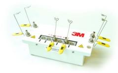
In a hot melt oven a fiber connector is heated up until the glue in the duct of the connector is molten. The fiber tip is now inserted in the connector. Special holders for the fiber and fiber connector allow heating up and cooling down of the connector. When leaving the connector cooling down the glue becomes solid and the fiber is rigidly fixed to the connector.
