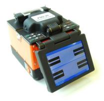
By a splicing machine the two bare fiber ends are arc fused. The two fiber ends are aligned by the splicing machine automatically. On the monitor screen of the splicing machine the alignment and splicing process can be followed. In a last step a splice protection sleeve is slid over the splice and heated until the sleeve shrinks and builds a firm protection against bending and tension.
